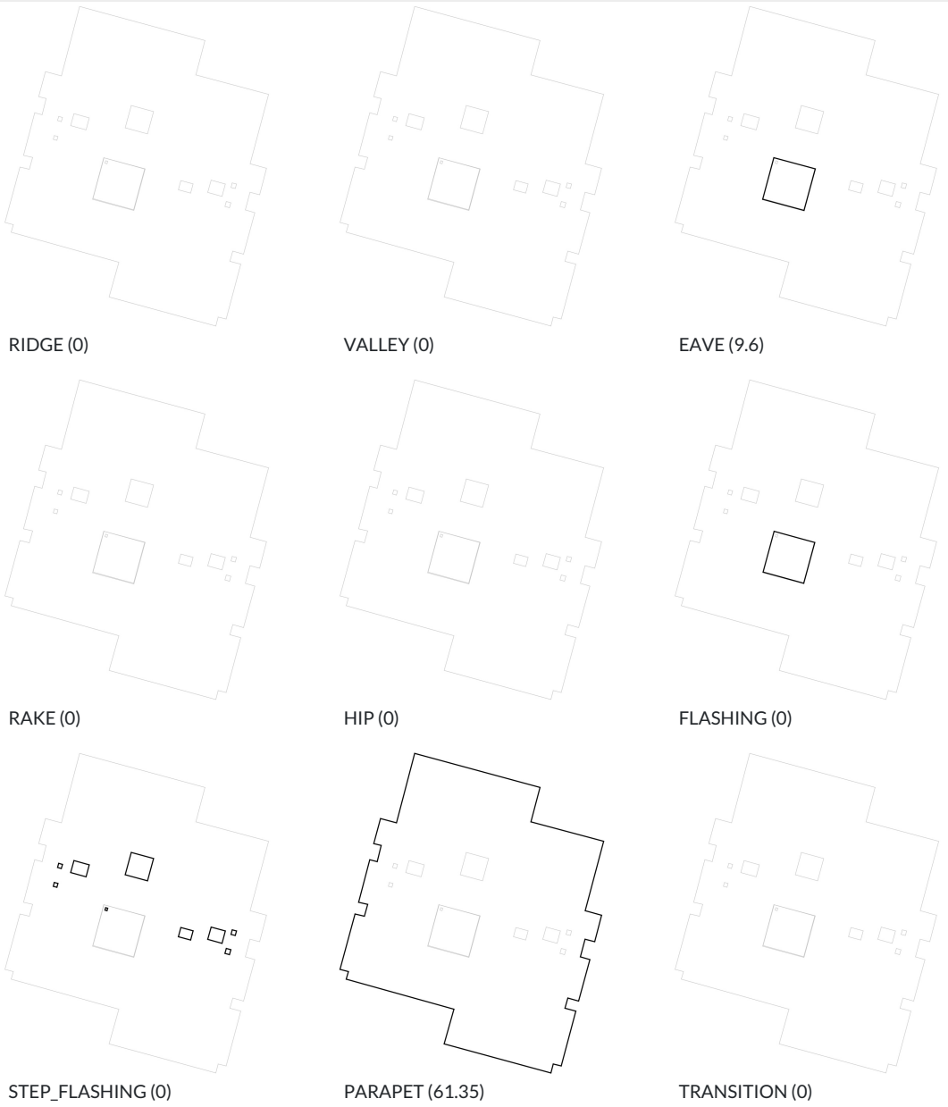
Figure 6: Roof Edge Classification (units: meters)
